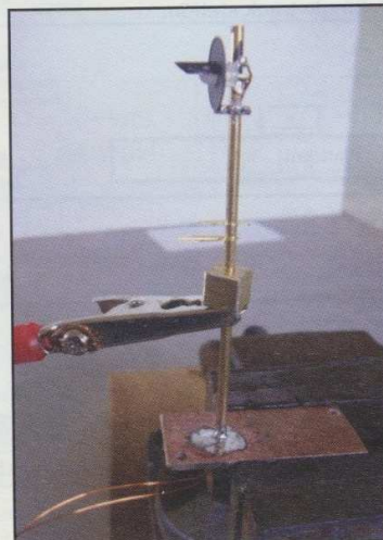
Fig 5 Holding mast in vice to solder.
