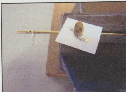
Fig 4 Solder shield to disc and U-shaped wire to mast.
