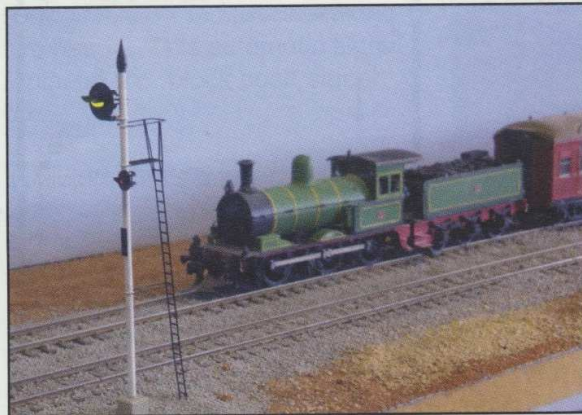
Fig 8 Automatic signal with fixed red marker.
